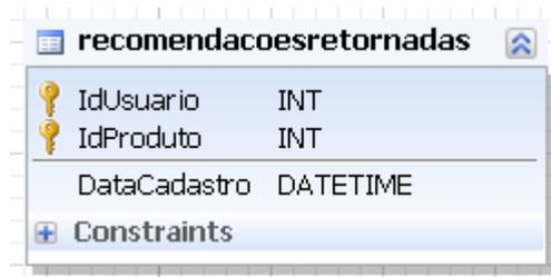
The image shows a screenshot of a database table structure for a table named 'recomendacoesretornadas'. The table has three columns: 'IdUsuario' (INT), 'IdProduto' (INT), and 'DataCadastro' (DATETIME). The first two columns are marked with a key icon, indicating they are primary keys. There is also a 'Constraints' section at the bottom of the table structure.
