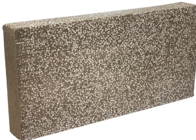
Figura 9- Concreto leve com EPS.
