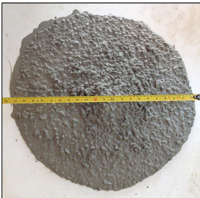
Figura 16–SlumpFlow Test
