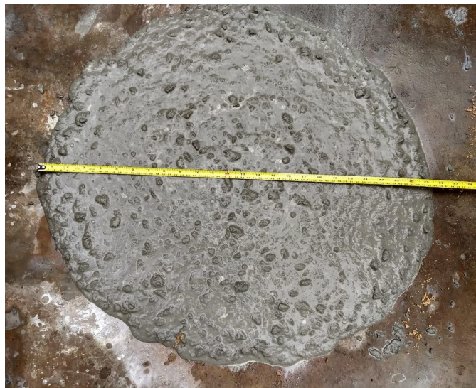
Figura 14 – Slump Flow Test.
