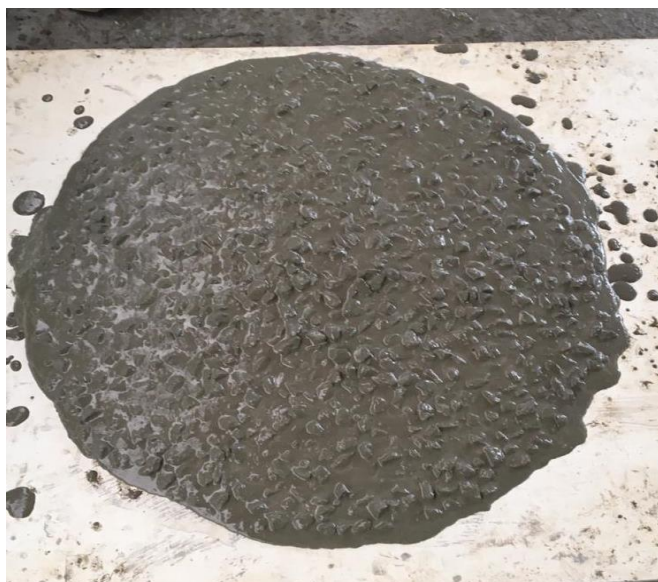
Figura 15 - Slump Flow test TR15% Intermediario.
